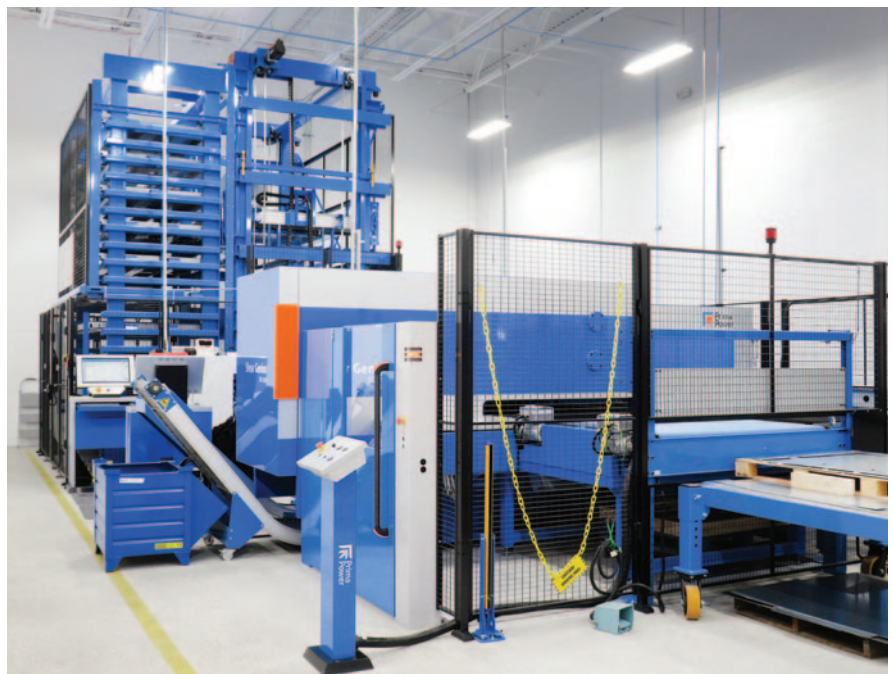
The Shear Genius SGe CNC punch-shear combination machine features an updated servo-electric 30-metric-ton punching machine with 1000-hits/min. stroke speed, 250-rpm index speed and 150-m/min. sheet-positioning speed. The right-angle shear has a servo-electric actuation system, which makes shear movement quick and fully CNC-controlled. The 10-station Combo Tower allows JST to store several gauges of galvanized cold-rolled steel, stainless steel and aluminum.
